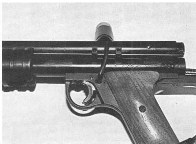
The Auto-Trigger is one of the most popular add-ons supplied for Sheridan airguns, but it won't fit on Mag-68s because of the factory direct-feed system.
